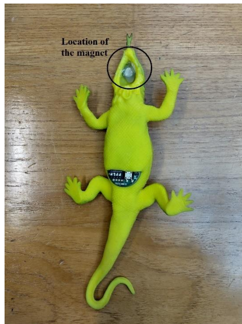
Figure 3518: Placement of magnet in the lizard's mouth
